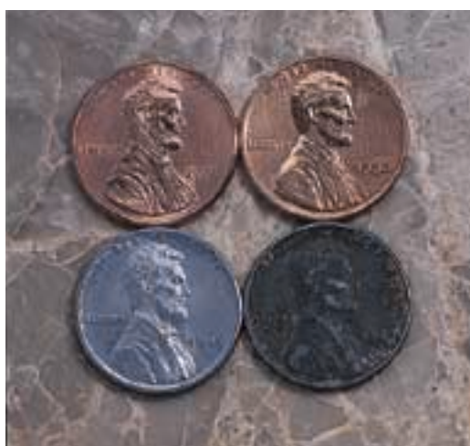
Figure 2 Zinc-copper and copper pennies (top); “new” and corroded zinc-steel pennies (bottom).
